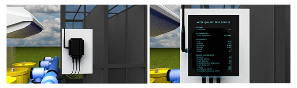
In the Genesis® IoT Blockchain solution, Arduino is used as the core controller running on a LINUX kernel. The temperature sensor, conductivity sensor, turbidity sensor, dissolved oxygen sensor, Ph sensor value are automatically calculated at the completion of every water treatment batch. Then the Arduino IoT device sends and stores the water quality data to the blockchain via its inbuilt Internet connection for safe storing and analysis.
